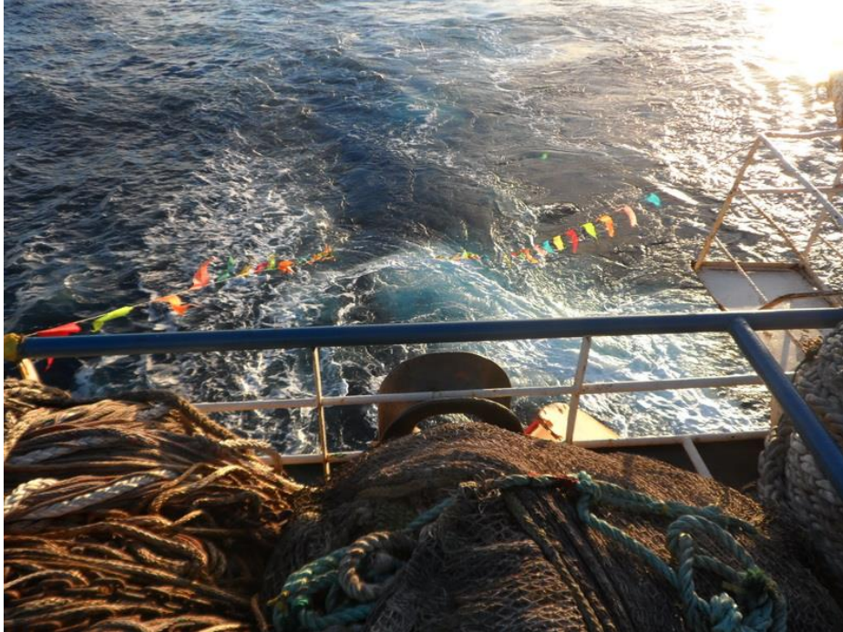
Figure 9a. Bird scaring lines attached to the stern of KAI FU HAO
