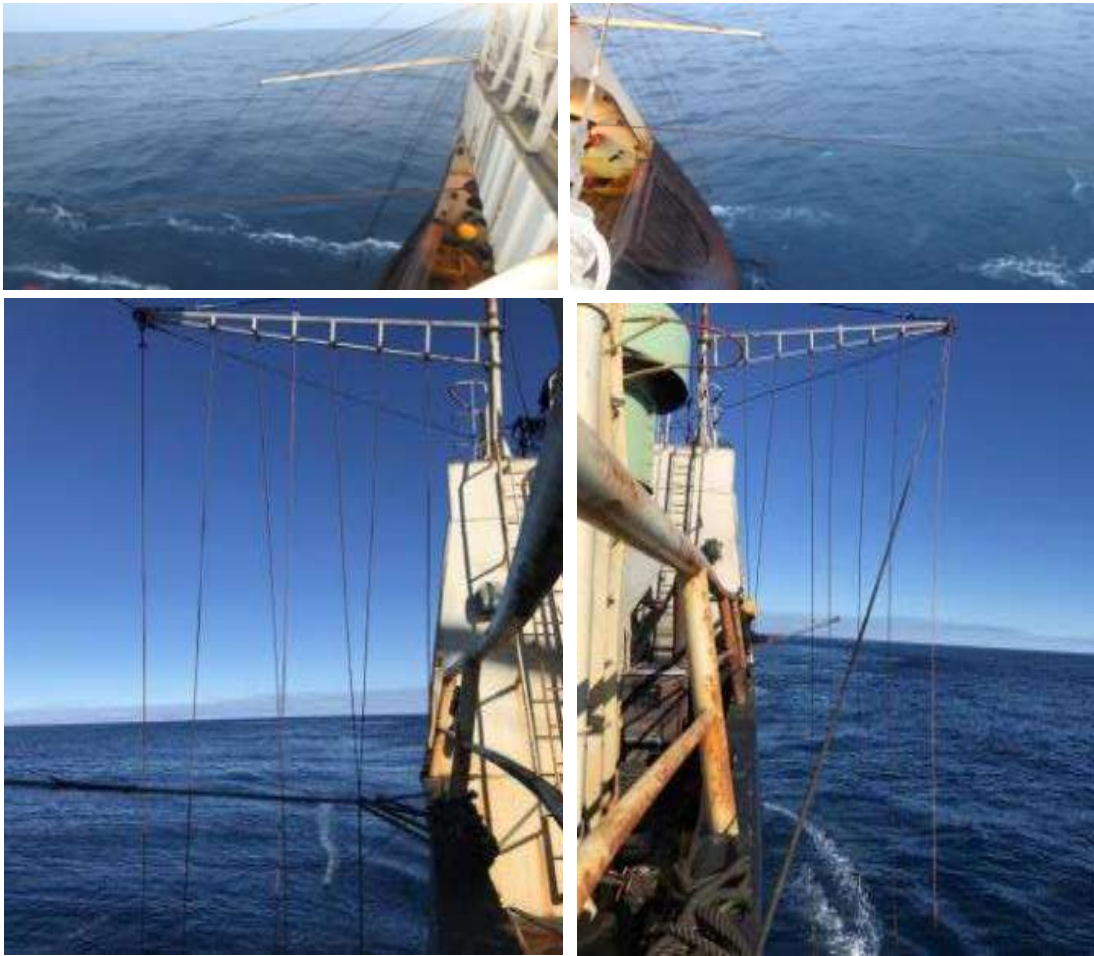
Figure 6. Photographs of setting up the bird baffle on vessels.
