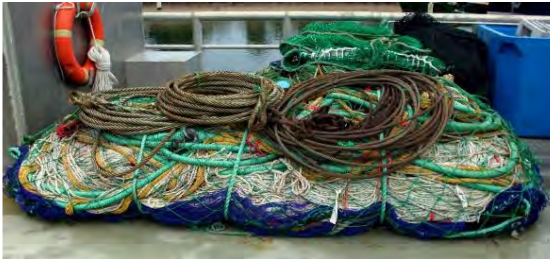
Figure 7: Wrapped wire rope used as footrope (top) and typical midwater trawl with light ground gear (bottom) used by New Zealand-flagged vessels when targeting alfonsino. Footropes can also be constructed using chains. Photos courtesy Talleys Ltd.
