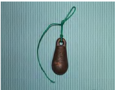
Figure 8: Hydrodynamic shaped steel line weights, 6kg each.
