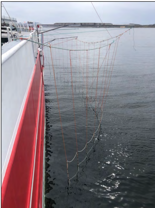
Figure 22: FV Tronio bird exclusion device (BED) around the hauling bay.
