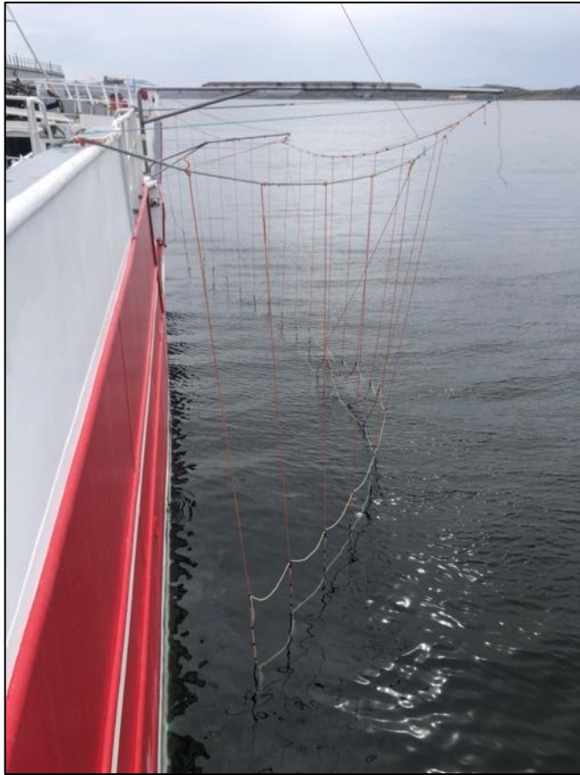
Figure 21: FV Tronio bird exclusion device (BED) around the hauling bay.
