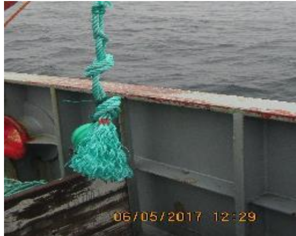
Figure 20: Towed device option 2, providing additional drag
