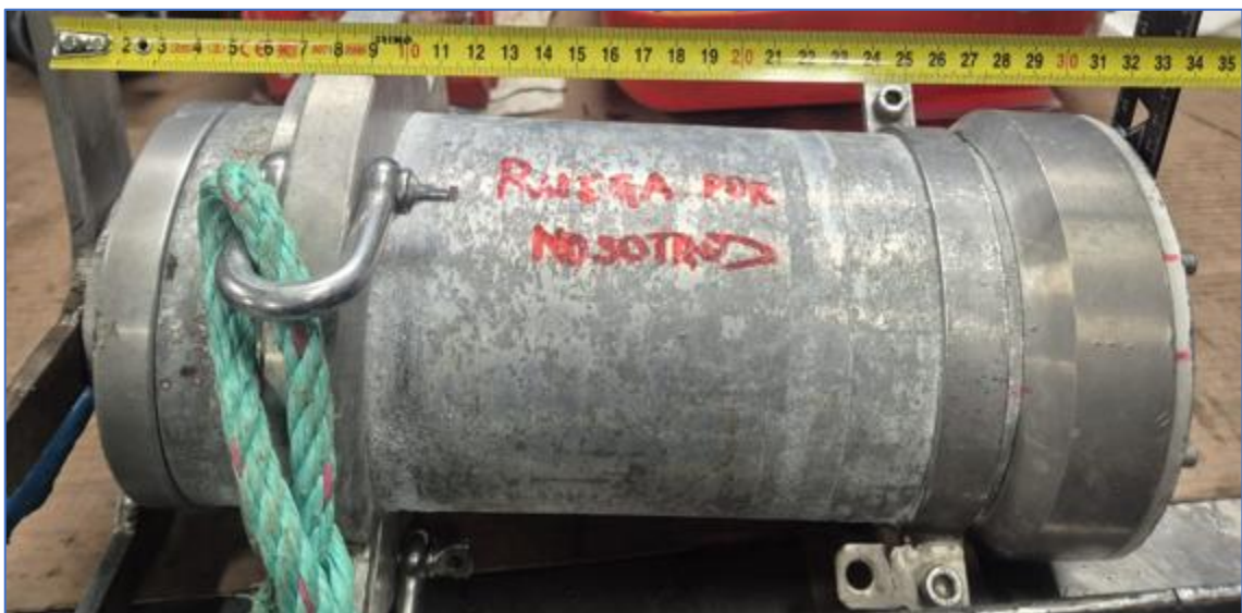
Figure 23: Benthic camera system deployed on longline. Camera system includes Akaso Brave 4 Pro ( https://www.akasotech.com/product/brave-4-pro ), battery pack, and LED light (2100 lum).
