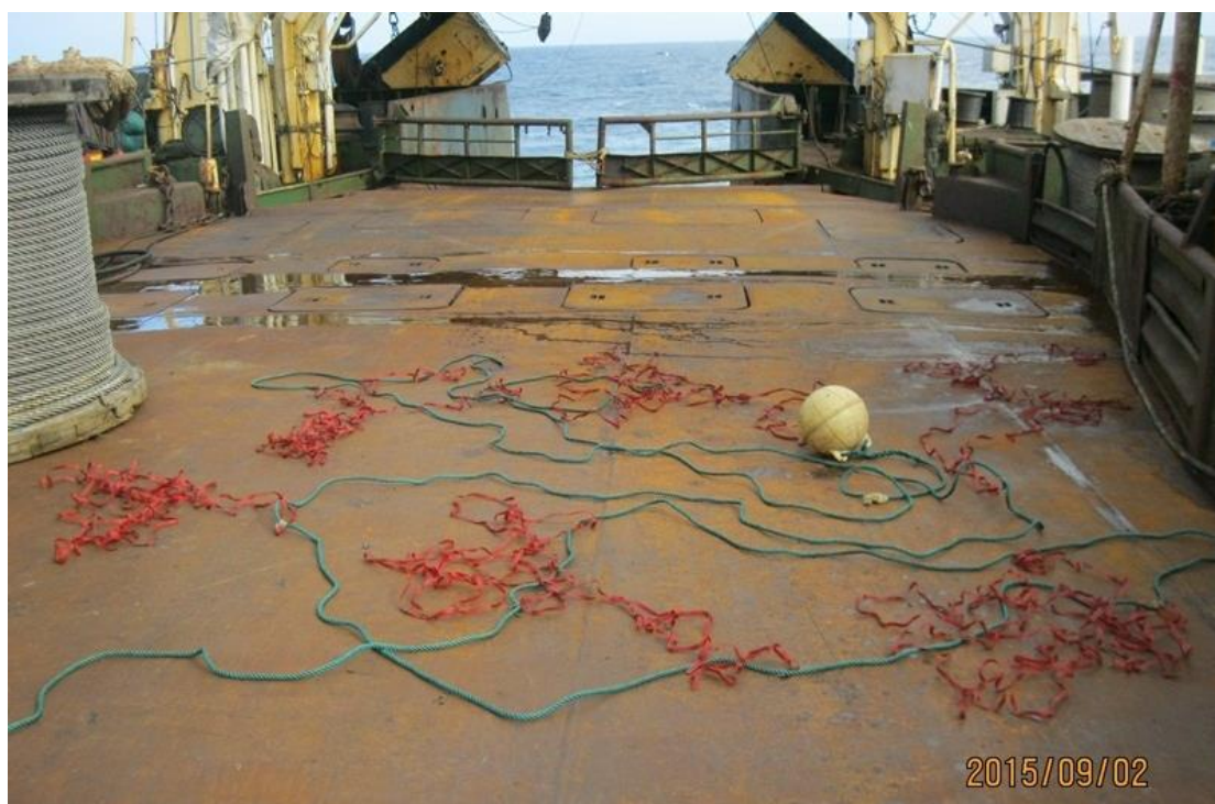
Figure 8 Bird scaring line of the Chinese trawler LONG TENG
