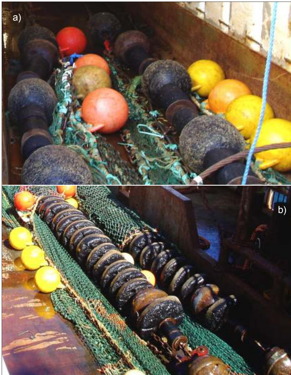
Plate 2. Alternate ground-gear configurations used when deepwater bottom trawling for species such as orange roughy and oreos showing ground-ropes equipped with a) 50-60cm rubber bobbins separated by rubber spacers, and b) with more closely spaced 60-80cm 'rockhopper' rubber discs plus leading end steel bobbins.
